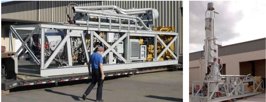
Figure 4, The ce25 is mobile and modular – once onsite the system can be assembled and operational within 48hrs.
